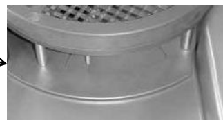
Photo 2. Scraper position which allows the demounting of the blade
