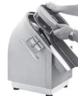
Fig. 10 Fixing the cube set with puller
