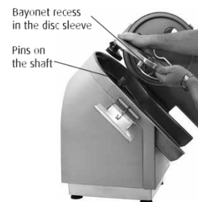
Fig. 8 Fixing the discs on the shaft
